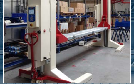
Cross-beam available for lifting under carriages and chassis
