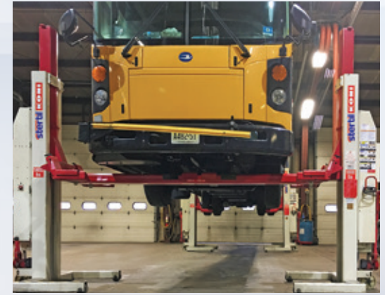
A Low Profile Crossbeam hoists a school bus allowing wheels-free access
