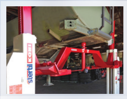
A Kingpin Crossbeam supports a military trailer on Mobile Column Lifts
