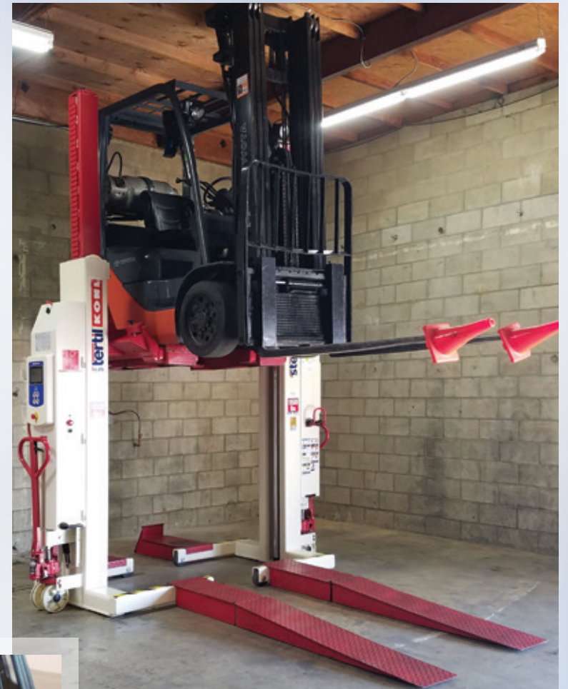
A Four-Wheel Forklift Adapter Kit on Mobile Column Lifts easily supports a forklift
